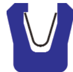
EC-External Face Cantilever Spring
